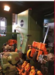
The traditional centreless machines for grinding and polishing tubes, bars and cylindrical parts, for small-medium productions, available in various configurations, both manual and automatic, for meeting the different working requirements.
